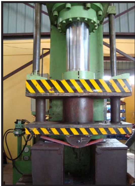
Clamps being hot formed in 150T press
