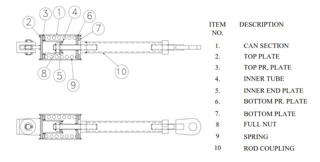
The construction is fairly simple, the unit has 2 pressure plates one on either side of the helical coil compression spring connected by a single piston rod.
